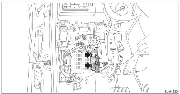
3) Remove the accessory relay (push button start) (A) from the relay and fuse box.
